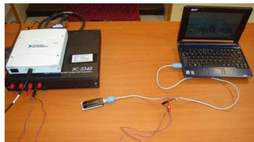
Figure 3 Dlink DWA-110 connected with NI's DAQ
